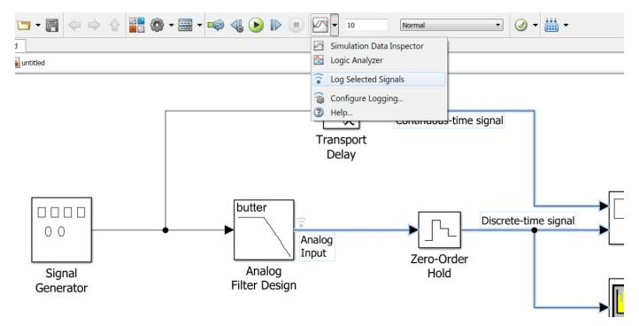
To visualize data in the Logic Analyzer, you must enable signal logging for the model. (Logging is on by default.) To enable signal logging, open **Model Settings** from the toolstrip, navigate to the **Data Import/Export** pane, and select **Signal logging**.
