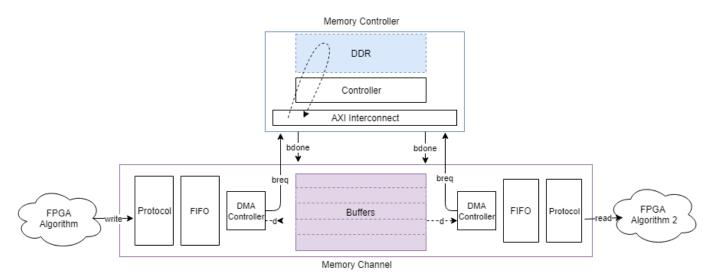
• **AXI4-Stream Video FIFO** – Model a connection between two hardware algorithms through external memory. This channel structure is similar to the **AXI4 Stream FIFO** configuration, but the writer and reader are using the MathWorks streaming pixel protocol, along with a back-pressure signal. For more information, see "AXI4-Stream Video Interface".
