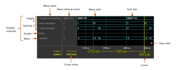
By default, when your simulation stops, the Logic Analyzer shows all the data for the simulation time on one screen. If you do not want this behavior, clear **Fit to view at Stop**. This option is disabled for long simulation times.
